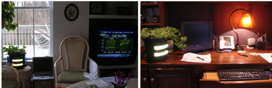
Fig. 3 Ambient Plant: Lights on plant pot glow in real-time when presence is detected on paired clock in other home
